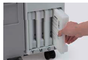
Simple ink cartridge replacement
